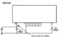
Be sure to evaluate it under the condition that it is mounted by your product. Especially, Confirm whether output current never exceeds a maximum standard with current probe.
